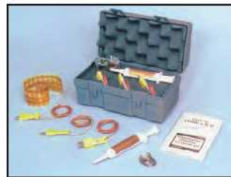
PAK-6 temperature profiling kit
